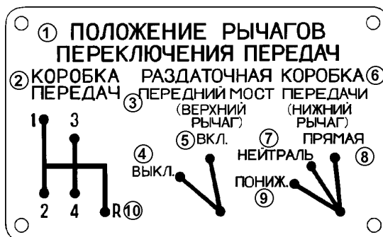
Fig.12. Instruction Plate. "Positions of Transmission, Front Axle and Transfer Case Shift Levers":
