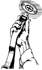
Fig. 74. Fitting suspension strap in place
